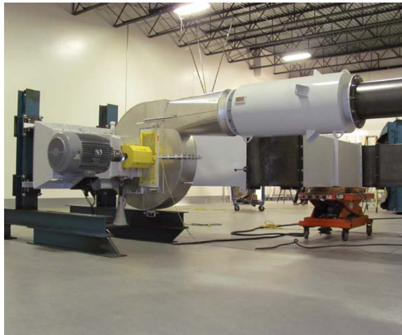
AMCA 210 Air Performance Testing
