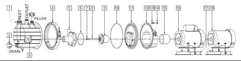
**NOTE:** When replacing impeller bushing in the field: The plastic bushing must be bored to size after they have been pressed into the impeller. Bore to 0.378/0.381 I.D. The carbon and ceramic bushings are to finished size and do not require boring. When attaching drive magnet to the motor shaft, position the face of the drive magnet 49/64 inch above the face of the motor bracket. When reassembling "V" retainer clamp, tighten down to 100-inch pounds.
