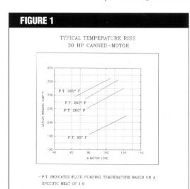
Typical temperature increase in motor windings
